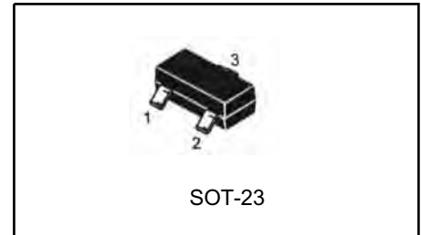
SOT-23 1: Ref; 2: Cathode; 3: Anode
